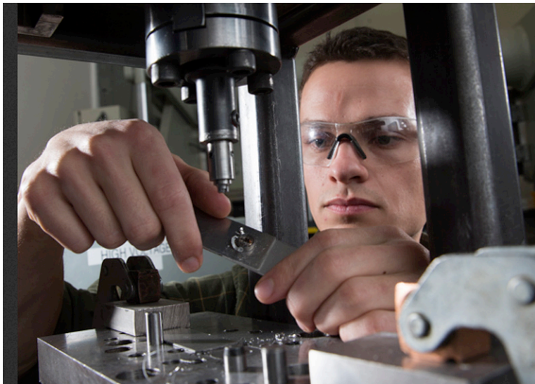
BYU manufacturing systems grad student Lile Squires bonds metals together with friction bit joining, a process that may help in developing lighter cars.
