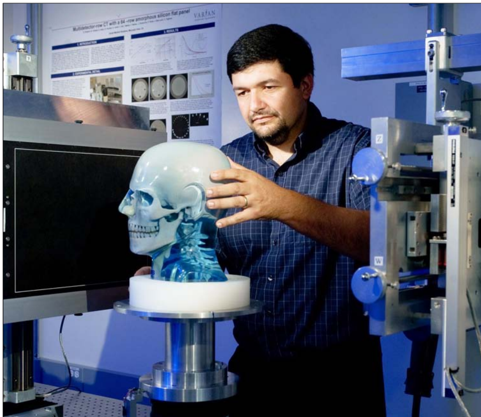
A Varian Medical Systems technician tests a flat panel image detector using an anatomically correct figure of a human head. The California-based company's flat panels are manufactured in Salt Lake City, the headquarters for manufacturing Varian's X-ray products and where the company has broken ground on an expansion project that will add 135,000 square feet and lead to 1,000 new full-time jobs over the next 20 years.
