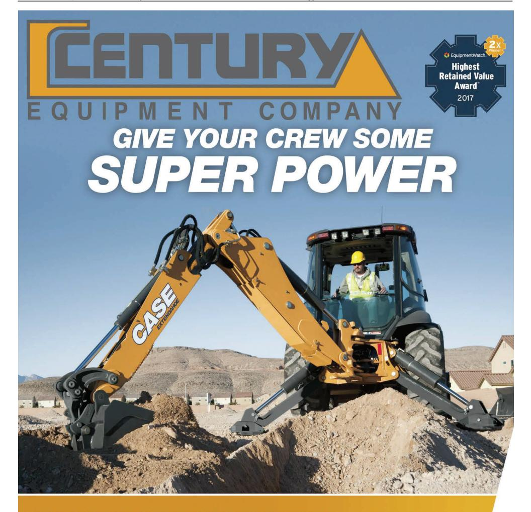
IMPRESSIVE IMPROVEMENTS TO AN ALREADY AWARD-WINNING MACHINE. An improved Pilot Control hydraulic system gives the 580 Super N greater feel and responsiveness for multi-function movements or precision work. An enhanced torque converter provides more pushing power under load and acceleration around the site. And new externally adjustable Extendahoe® wear pads make it easy to stop slop in the dipper. It's the same Super N, now with more super. Learn more at CaseCE.com/580SuperN
