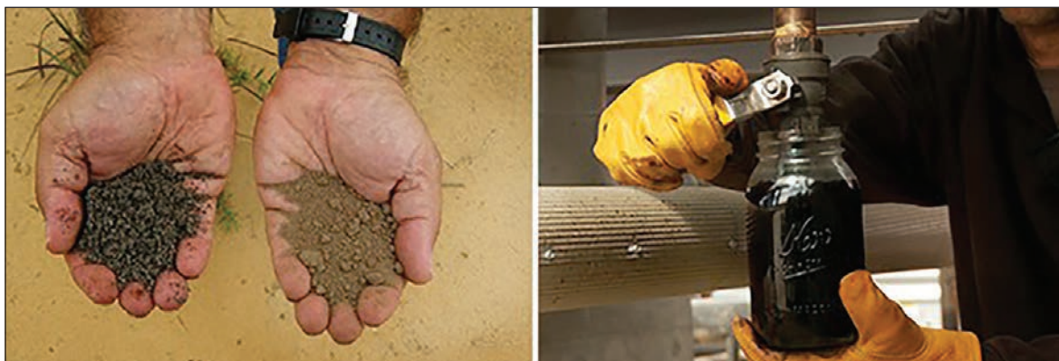
(Left) A technician at Petroteq Energy's oil sands refinery near Vernal demonstrates the difference between the oil sand going in and clean sand ready for recycling coming out. At right, a sample of the salable crude oil the plant produces is drawn for testing. Petroteq Energy Inc. photos.
