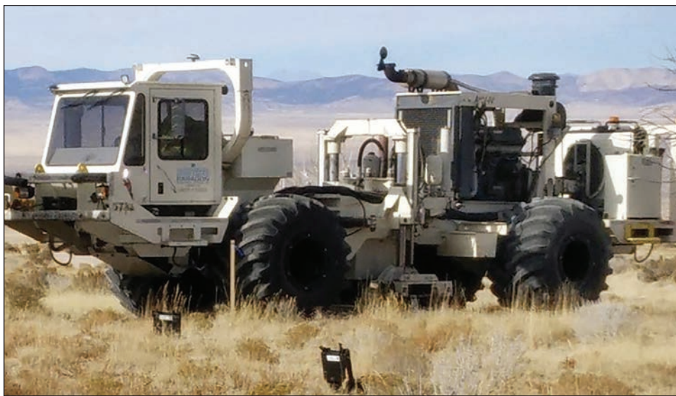
As part of the investigation and site evaluation for the awarding of a Frontier Observatory for Research in Geothermal Energy research grant from the Department of Energy, truck-mounted vibrator plates probe the earth near Milford with seismic waves to determine suitability for thermal energy development. The Beaver County site was selected over four other western United States sites for $140 million in funding.
