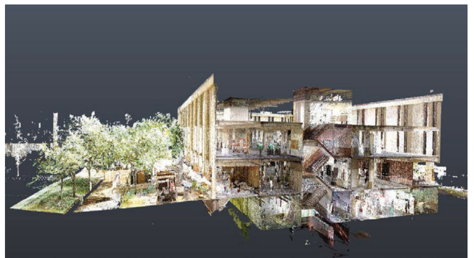
LiDAR Scanning and Building Information Modeling were used to map critical systems inside the building.
