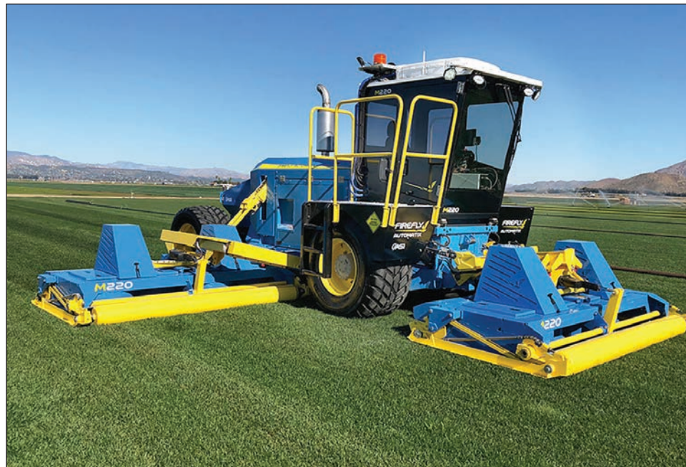
FireFly Automatrix Inc. of North Salt Lake demonstrates its M220 mower, an unmanned self-propelled, hybrid turf mower driven by controls and software developed by Autonomous Solutions Inc. of Mendon. The vehicle was introduced and demonstrated in February at the Turfgrass Producers International Conference in Tucson, Arizona.
