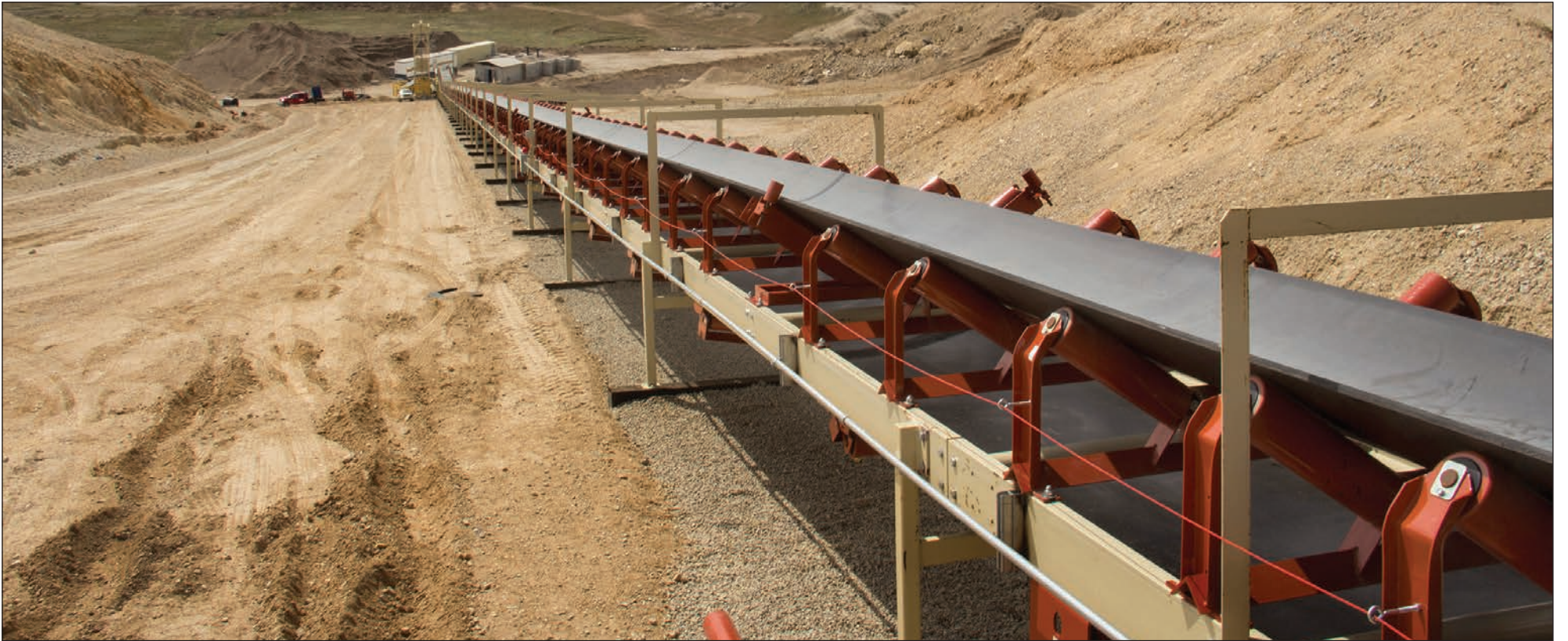
When product is going downhill at the Geneva Rock quarry, gravity moves the conveyor belt system with enough force to generate electricity that can be used to power other parts of the operation.
