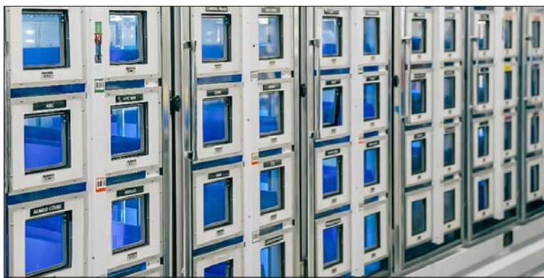
ARUP's sort-to-light system enables employees to distribute specimens quickly and efficiently. They scan a bar code on each specimen to prompt the compartment where the specimen should be placed to light up.
